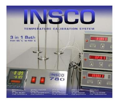
Taking into consideration our immeasurable experience in Metrology, INSCO has developed the Ultimate Calibration Machine. Our 780 Model, also known as the "3 in 1" enables calibration labs to perform test at 3 different set points simultaneously with a single Dry Well.
